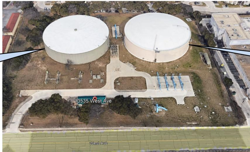
Existing 5 MG Steel GST to be Demolished and Replaced with new Prestressed Concrete GST
